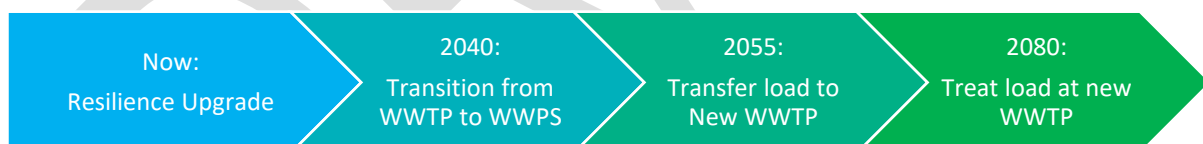
Figure 3-24: Athenry WWTP Recommendations
